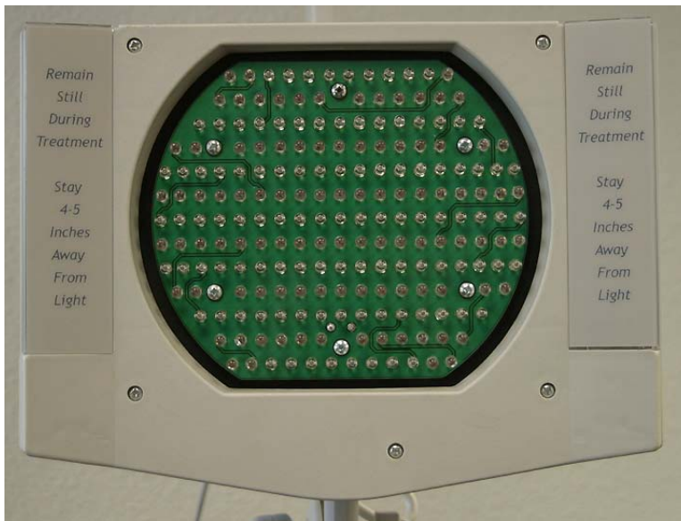
Figure 1. The face of the Dermillume Healing Red Lamp with 98 red and 104 near infrared LEDs.
